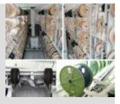
Integrated dual unwinder for quick cable change
